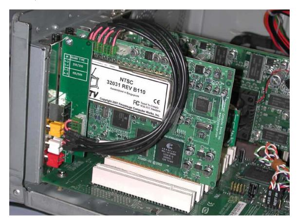
For the WinTV-PVR-250/350 (250 shown above) connect the jumpers to pins 1-2 & 3-4 on the A/V Cable Set between the A/V header and audio/video inputs.
