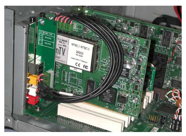
For the WinTV-PVR 150/500 (150 MCE shown above) connect the jumpers to pins 2-3 & 4-5 on the A/V Cable Set between the A/V header and audio/video inputs.
