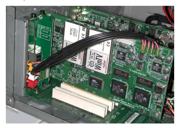
For the WinTV-PVR 150/500 (500 MCE shown above) connect the jumpers to pins 2-3 & 4-5 on the A/V Cable Set between the A/V header and audio/video inputs.
