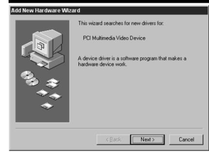
**4a.** When re-starting Windows for the first time after the WinTV board has been installed, the **Add New Hardware Wizard** will appear.
