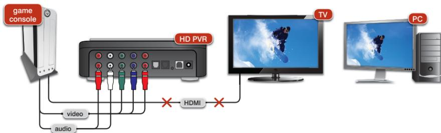
**Note: if you have an HDMI cable connected between your game console and your TV set, - disconnect it. Instead, use the Pass Through video connection (see No Delay Video Pass Through below).**
