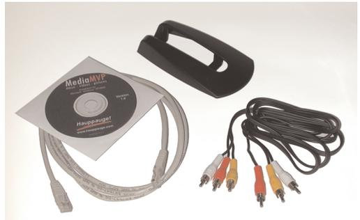
\* **Note:** you can purchase longer ethernet cables at most computer retail stores. Cat5 cable, as the cabling is commonly called, is available to lengths of 300 ft.
